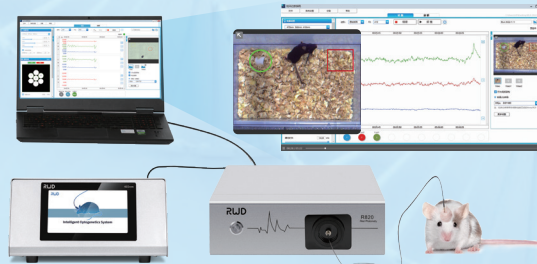
To realize light stimulation and signal acquisition for the same site
